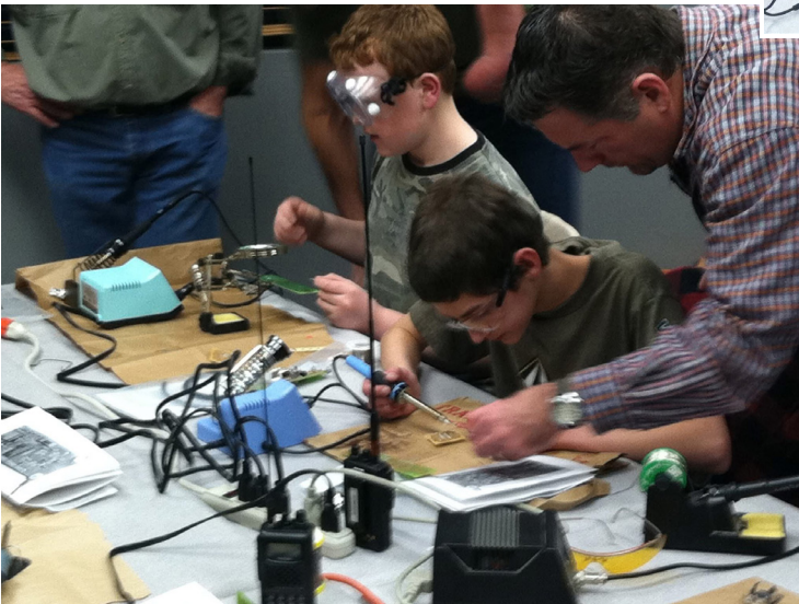
James KDØMFØ helps Ethan KDØMFP solder a component onto a TDOA device printed circuit board.
