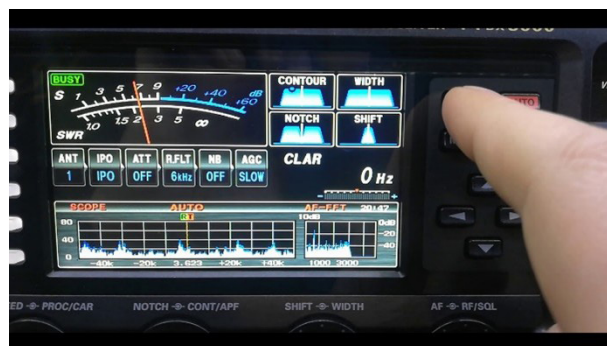
Figure 3: The noise blanker (NB) control is usually found on the front panel or menu.
