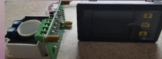
DC meter with current shunt
