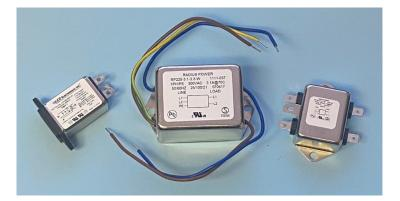
Filter body MUST be bonded to chassis and located near the mains input for common mode filtering.
