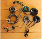
Ideally, these should be located at both the antenna and radio
