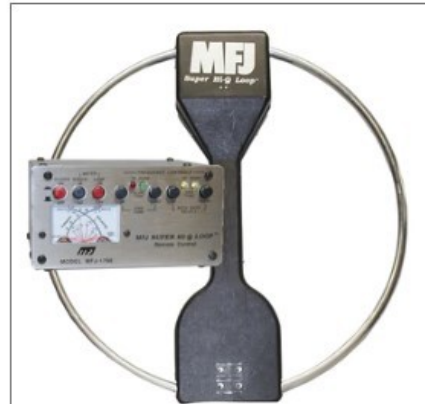
MFJ-1786X, SUPER HI-Q LOOP, 36~ DIA, 10-30 MHz, 220VAC
